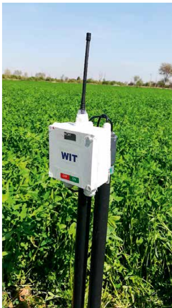
These sensors assist farmers in making informed irrigation decisions, allowing them to achieve increased crop yield at reduced irrigation cycles
